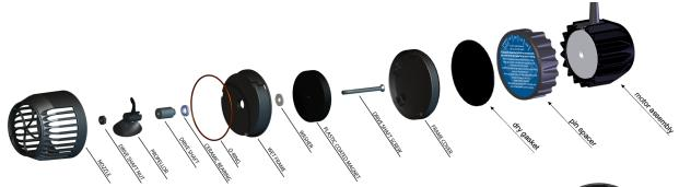
To remove the nozzle from the wet frame, remove the entire wet half of the pump from the aquarium and place it on a non-metallic surface. Gently but firmly press down on the nozzle with your palm and twist counter clockwise. The nozzle should become free of the wet frame. It may then be cleaned of any obstructions.
