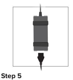
1. Strap the power supply back into the Assembly and it is ready for use.
