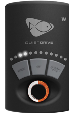
Driver shown in Configuration Mode Main Menu, sitting on Night Mode Speed option.
