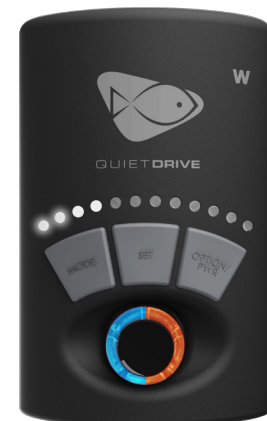
Driver shown here in Auto-Dim Time Configuration Mode Setting, showing that it is set to 1 minute and default being disabled.
