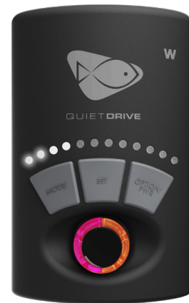
Driver shown here in Night Mode Time Configuration Mode Setting, showing that it is set to a 6 hour night and default being a 10 hour night.
