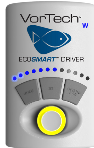
Illustration above shows an EcoSmart Driver in Random Mode (Yellow Control Dial). The first and second brightly illuminated LEDs show that this driver is set to Reefcrest Random along with the dim LEDs showing the speed setting.
