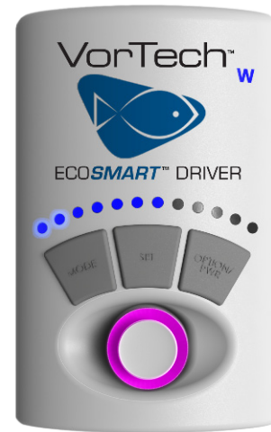
Illustration above shows an EcoSmart Driver in EcoSmart Mode (Purple Control Dial). The first and second brightly illuminated LEDs show that this driver is set to EcoSmart TSM along with the dim LEDs showing the speed setting.
