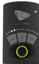
Lagoonal Random Mode simulates a low-energy lagoon environment. It is indicated by a yellow control dial and the third and fourth LEDs illuminated. The control dial is used to set the maximum speed of this mode. The speed of the pump is changed slowly to recreate the gentle currents of a lagoon.
