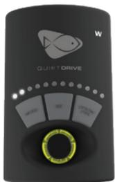
Reef Crest Random Mode simulates a high-energy reef environment. It is indicated by both a yellow control dial and the first two blue LEDs illuminated. The control dial is used to set the maximum pump speed during this mode. The pump will change speed frequently and drastically to simulate crashing waves and surging tide.
